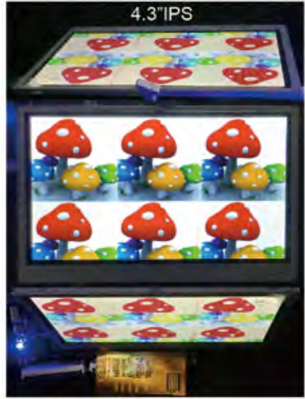
IPS TFT 4.3 inch 480x272 IPS glass 450 nits brightness backlight or higher
